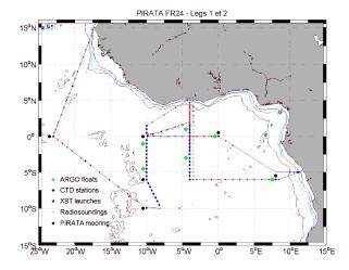
Major issues & problems during this cruise were: i) the CO2 sensor at 6S-10W does not work; ii) one ARGO profiler failed after its deployment (close to the PIRATA SEE location); iii) some problem with the wind sensor at 6S-8E from May 24<sup>th</sup> (*Bad data transmitted*; *to be checked*).
