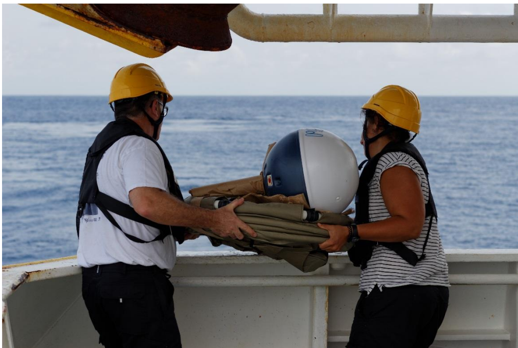
Deployment of a Surface Velocity Profiler equipped with a Barometer (Picture: Y.Gouriou, IRD).
