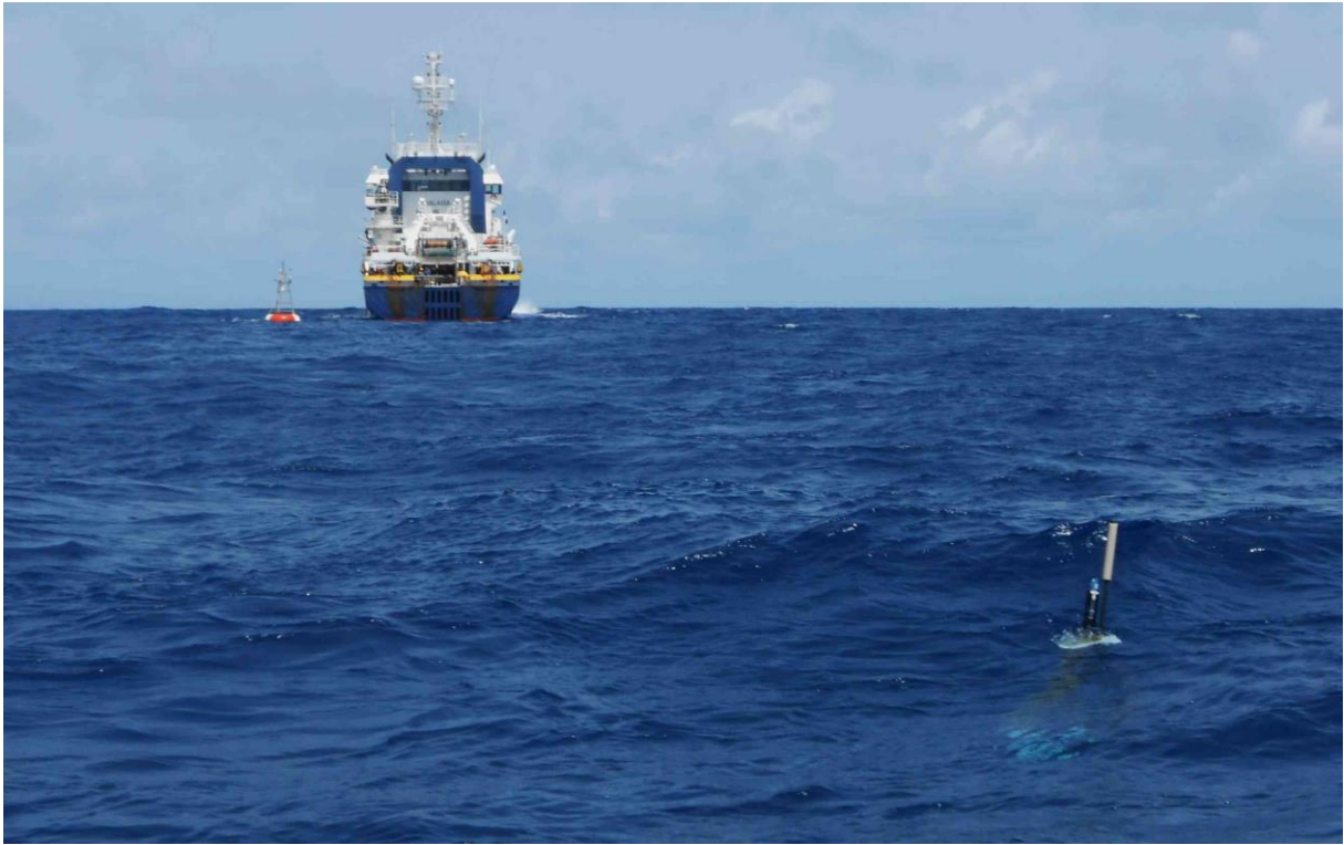
A Deep-Argo profiler just after its deployment at 10°W-0°N, close to the just serviced ATLAS buoy observed on the left of the R/V Thalassa (Picture: B.Bourlès, IRD).
