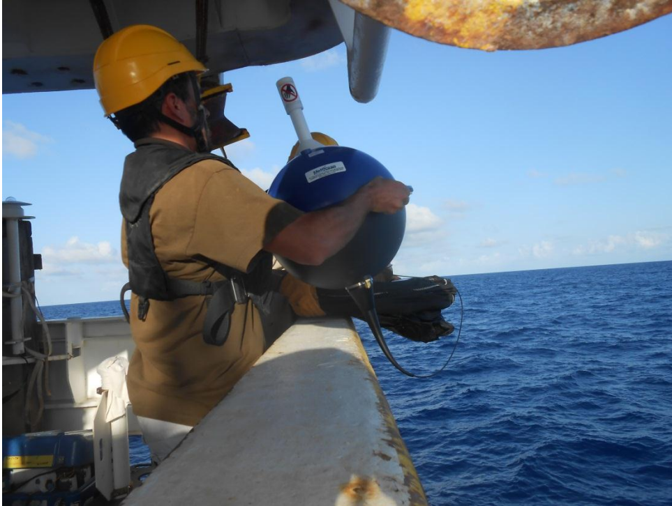
Deployment of a Surface Velocity Profiler equipped with a Barometer (Courtesy: B.Bourlès, IRD).
